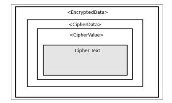
Figure 2.1: Enveloping encryption
