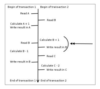
Figure 2.3: Example of concurrent transaction processing
