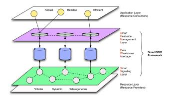
Fig. 1. SmartGRID architecture overview
